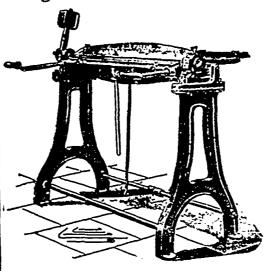
This machine will foll edges from onesixteenth of an inch to 1 inch flat for grooving, or any other angle required: also a round edge for straight wring, and a doubl-fold or metal clips for almanaes, show-eards, e. As an angle bender it will take any length of sheets, and turn either squares or round corners for canisters &c.
