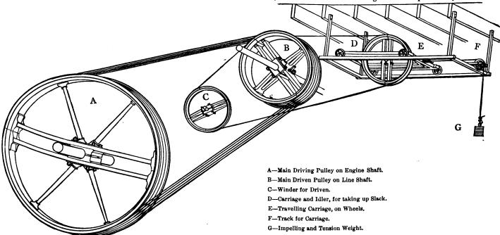
The illustration, Patent System of manilla ropes and grooved hardwood pulleys. Transmissions similar to the above are now in use at the works of the following well-know manufacturers in Toronto:—
