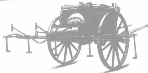
shown in illustration, and one horse, you can rid your potato-fields of the blight and the bugs at the rate of one acre in 20 minutes. Has non-clogging nozzles, 12-gallon air-tank; 100 lbs. pressure guaranteed with 12 nozzles open. Agitator clean-out pressure into tank, and nozzle protector, controlled from seat. Can be fitted for orchard, vineyard and grain crops. For one or
