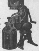
Note the heavy compact construc-tion and convenient height of supply-can and discharge spouts. The top of the supply-can is only 3½ ft. from the floor,
