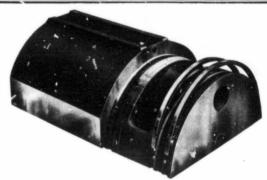
Among the many valuable features of the Gould Balance Valve which are always appreciated by the operator, is the ease of handling the engine, saving of the valve gear, saving of wear and tear on engine, and lack of probability of a single cylinder engine stopping on the center.
