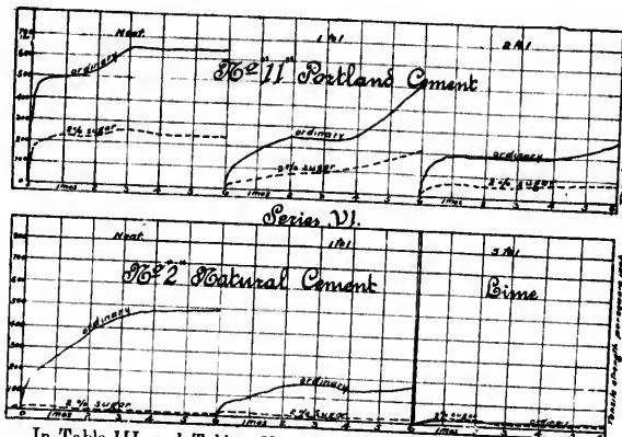
In Table III, and Table IV, the per cent. of evaporation in 2 days is again given, and diagrams are plotted showing the relation between the tensile strength and the weight of the dried briquettes in the pressure tests, and also other diagrams showing the product of tensile strength and evaporation plotted on a base of weights of briquettes.
