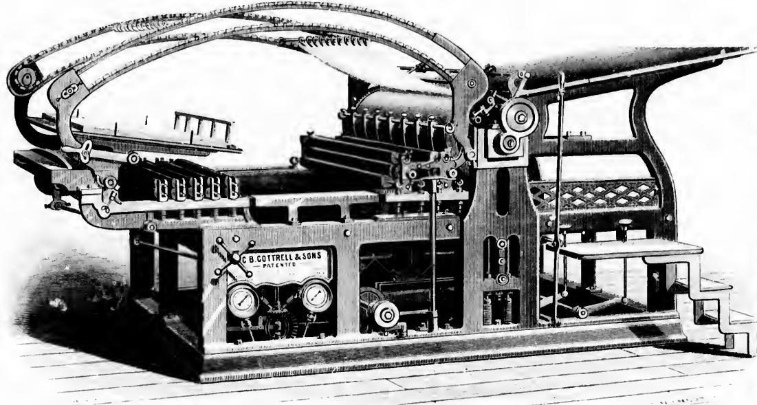
THE above engraving represents our new series of TWO-REVOLUTION PRESSES. This machine has been entirely reconstructed and strengthened throughout, and many of the mechanical arrangements greatly simplified. The reconstruction has been rendered desirable because of our many improvements that have been placed in the best possible positions for convenience in working, and at the same time present an artistic design as a whole.
