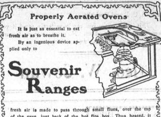
of the oven, just back of the hot fire box. Thus heated, it enters the oven and by a direct current of air the impurities and cooking odors are carried up the chimney.
