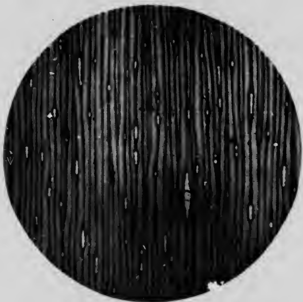
PLATE 55. PINUS GLABRA . Tangential section through the spring wood showing the ordinary rays with terminal tracheids and with the thin-walled parenchyma all broken out; the interspersal of the tracheids and their general predominance; the structure of the low and rather broad fusiform ray, the thin-walled parenchyma cells of which have been broken out, leaving only a portion of the resin canal in the central tract together with the terminal tracheids. \times 46.8
