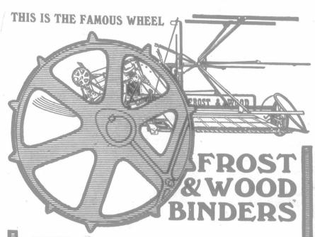
HE eccentric sprocket wheel on the Frost & Wood Binder prevents the "chug" and strain on team and machine you will notice in ordinary binders. What does this mean to you? It means your machine will last longer. It means swifter cutting—you reach the end of a big field before it is too ripe. It means well-compressed sheaves. It also means saved wages by shortening your harvest season.
