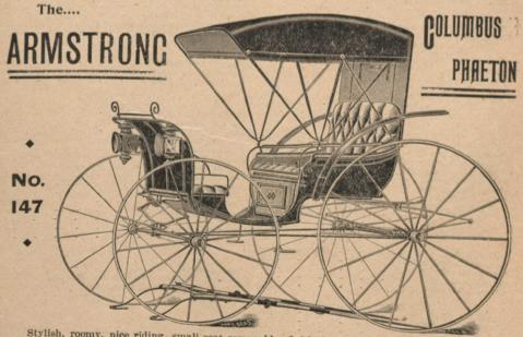
Stylish, roomy, nice riding, small seat removable, finished throughout with best material and workmanship. Spring cushion and spring back; full lined rubber or leather top; wing dash with lamps; B. Standard wheels  $\frac{3}{4}$  in. and 1 in. tire, steel axles. Price reasonable for a first-class job. Catalogue of all styles, and any particulars desired furnished freely on application.
