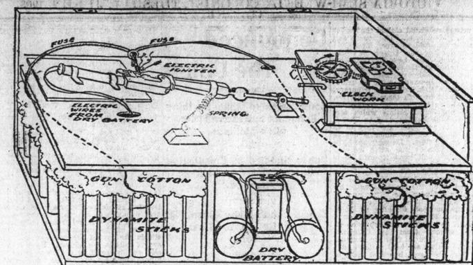
This is a diagram of the infernal machine which was intended to destroy the Umbria. It is said to be the most perfectly constructed instrument of destruction of the kind ever seen.
