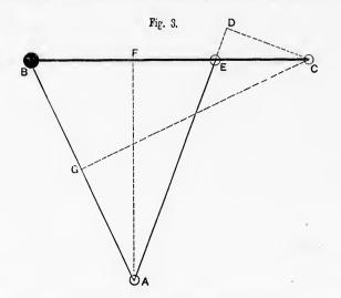
E, in which case the weight at E is to the actual weight at B as B C to E C. The centrifugal moment of weight B for any given number of revolutions is proportional to the radius BA times the line G C, drawn at right angles to BA through C. The centrifugal force of the resultant weight E is similarly A E times D C; D C being drawn at right angles to A E prolonged. According to the theorem,
