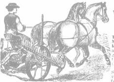
The Simplest, Lightest Draft and most Durable The Simplest, Lightest Draft and most Durable Mower made. It is almost impossible to stone the knives as we use 2½ inch sections, the finger-bar having a rolling or warbling motion allows the points of the guards to rise or fall and adapt itself to the unevenness of the seil without having to use the tilting lever. We make the "Warrior" with either 22 or 24 section knife.
