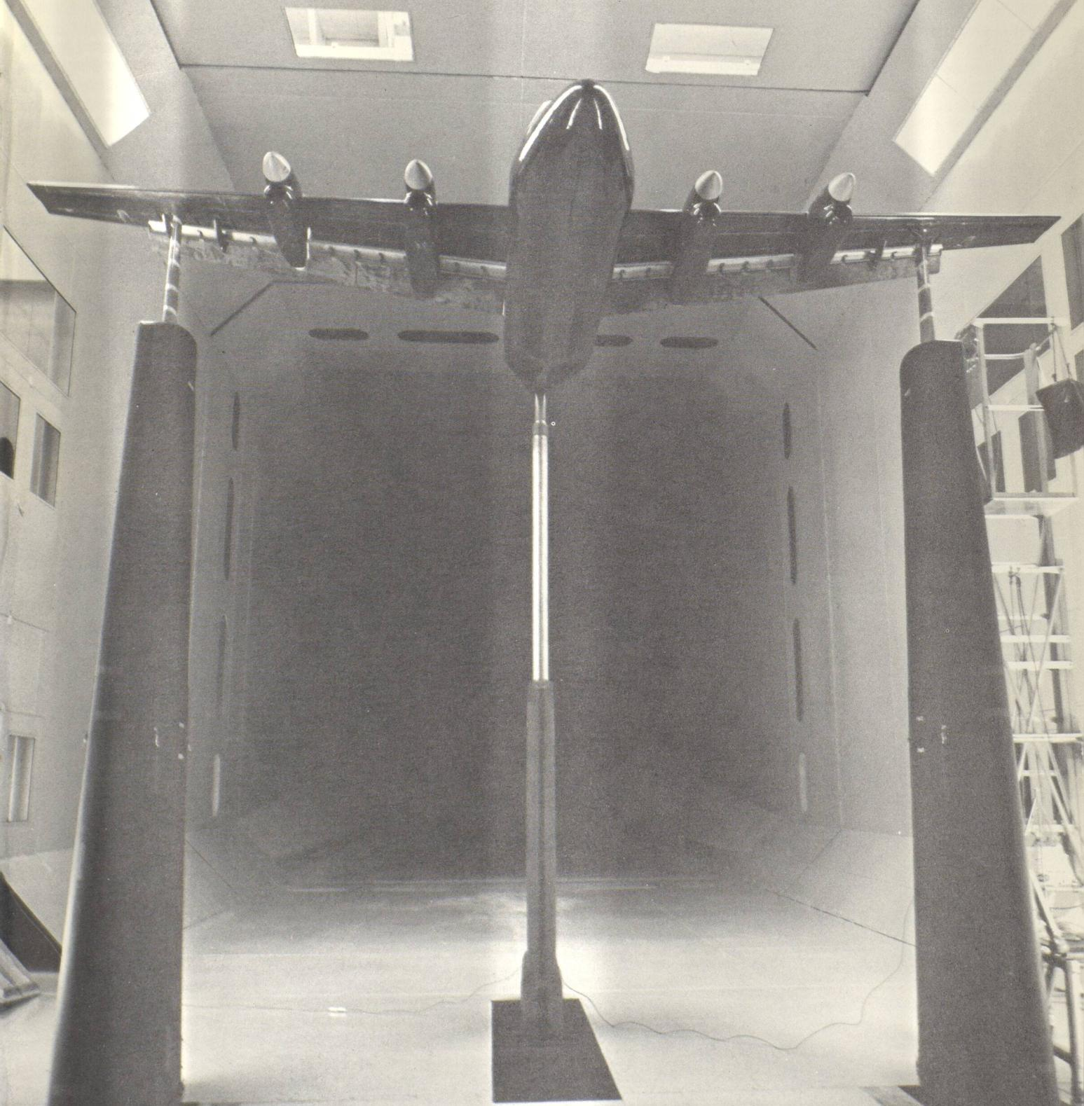
First model to be tested in the 30-foot wind tunnel is de Havilland Aircraft's DHC-7 airliner. The model rests on support struts linked to a six-component mechanical balance. The balance separates the total load into six parts — lift, side force and drag or thrust (if the model's four 100 horsepower electric motors are working); and the three moments of pitch, roll and yaw.
