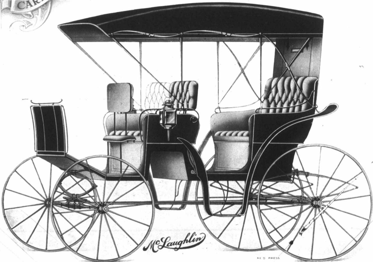
No. 497 Large Cut-Under Surrey, with Long Toe : Reversible Front Seats ; Three Spring Gear.
