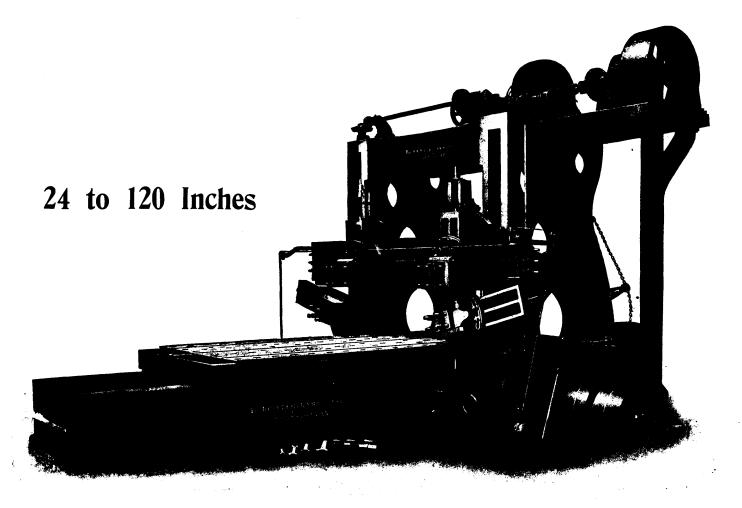
84-Inch Planing Machine-Motor Driven with Power for Operating Side Head.
