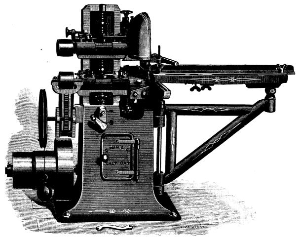
This is an entirely new style of Tenon Machine. The frame is east in one piece, and the working parts stand solidly on a pedestal, avoiding all vibration.
