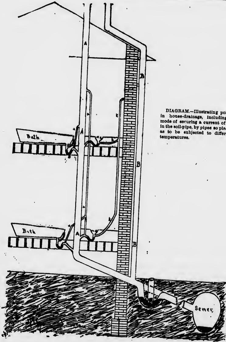
DIAGRAM.—Illustrating points in house-drainage, including a mode of securing a current of air in the soil-pipe, by pipes so placed as to be subjected to different temperatures.
