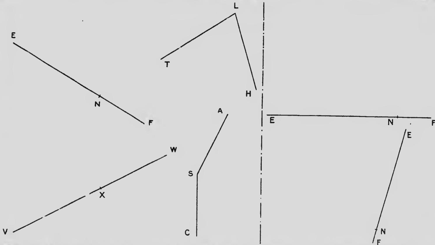
**PROBLEM 3.**—At a given point *N* in the given line *EF*, to make an angle equal to the given angle *TLH*.
