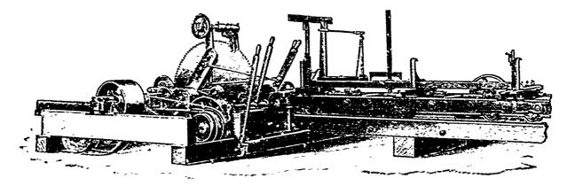
I make these mills with any number of Head-blocks spaced any distance apart. Equipped with Frost-dog, Knight dog, or Boss dog, Rope feed, or Rack and Pinion feed. With or without Over Log Saw Guide.
