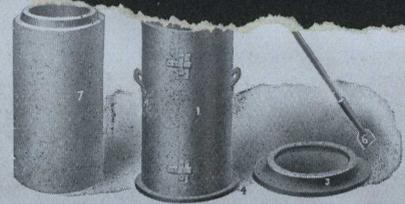
View of complete Mould for 1909, with section broken out showing bottom ring which makes telescopic joint. The Moulds, which are made of heavy steel plate, with three hinges and latches, make tile 30 inches long. Sizes from 4 inches to 48 inches. Write for new prices.
