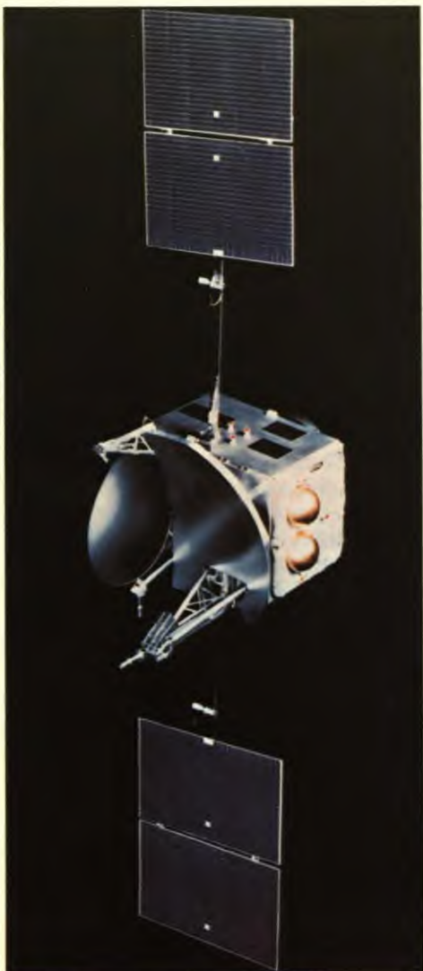
Anik B, a Canadian communications satellite launched in December 1978, makes 12 channels available for commercial domestic use. The satellite weighs 923 kilograms and is 1.8 metres wide and 11.3 metres high with its solar panels extended.
