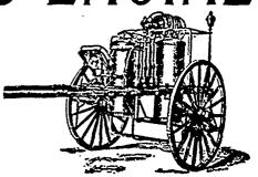
This machine is the most powerful fire fighter. It has two cylinders, 40 gallons capacity each. The combination of chemicals will not freeze, renders material with which it comes in contact non-inflammable, and will not corrode when not in use. For full particulars, write to the Bead Office of the Company at Kingston.
