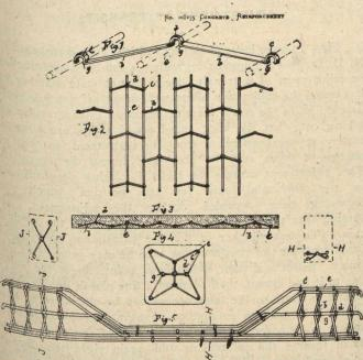
reinforcement work. The cut shows, first, the manner in which the bars are attached to the rods; next, the bars attached to rods and ready for the concrete. Fig. 3 shows a cross section of the floor after the concrete. crete is laid, while the remaining figures show the reinforcement in beams and columns. One of the claims made in favor of this reinforcement is that only plain,
