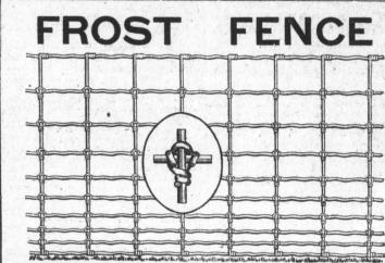
This fence is made in Canada enitrely of Canadian products. All the wires are full size true to gauge. Laterals and uprights are all No. 9 Hard Steel, well galvanized stock. Laterals are given a deep and continuous wave for "give and take." These coils or waves serve like a spring keeping the fence tight throughout all seasons and under all conditions. It is used by the principal farmers everywhere. The cost to you is no more
