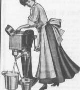
Tubular supply cans are low, steady, easy to fill and need not be removed to take the machine apart. The driving gears, and the ball bearing from which the bowl hangs, are enclosed, dust proof, self oiling,
