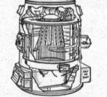
One of the reasons why the Kelsey can deliver more warm air than any other Heating System is based on the construction of the zig zag Heat Tubes or Sections.
