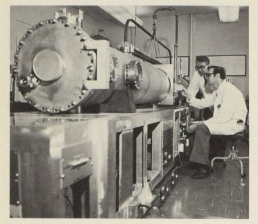
as the world's most accurate bientôt en service à la section clock in the Time and Frequency Section of NRC's Division of Physics and will form the basis for Canada's official time scale. Dr. Allan Mungall (right) was responsible for the overall design and was assisted by Mr. Herman Daams (left) and Mr. Ralph Bailey.
