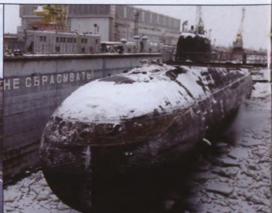
Nuclear-powered submarine in floating dry dock
