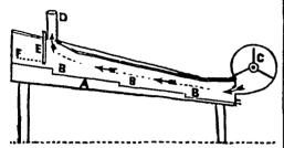
ference to the drawing, in which the principle of the operation and the various parts of the mechanism may be clearly seen. These last consist of a covered trough (A), with a series of steps (B) (B) on an inclined plane, a fan blower (C), worked by hand or any available power, a chimney or air duct (D), to carry off the warm and impure air, as shown by the arrows, a movable sluice or floodgate (E), to regulate the flow of the milk, a strainer (F) to remove hairs, &c., that might be in the milk.
