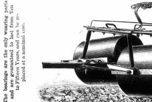
There is no axle shaft, no strain, and consequently no wear. It is easily ciled between the drums.
