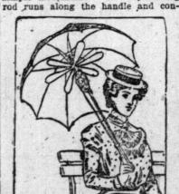
nects with a gear wheel connected with the wheel at the end of the fan, and is sent spinning by a single pull of a ring near the parasol's handle. The owner thus obtains shade and breeze at the same time.
