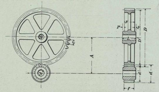
Machine Moulded Gears up to 18 feet in diameter without the use of patterns. Only necessary to furnish dimensions as shown in above cut.
