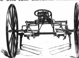
Knives can be Locked in any Desired Position.
