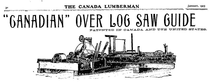
This Over Log Saw Guide is no longer in the experimental state. Any intelligent sawyer can handle them, and use much thinner saws, thus saving a large amount of lumber that is usually converted into saw dust. One of our leading saw manufacturers says : 'They will be a great help to any saw." I make them to fit on existing saw frames, and sell with or without saw rig as desired.
