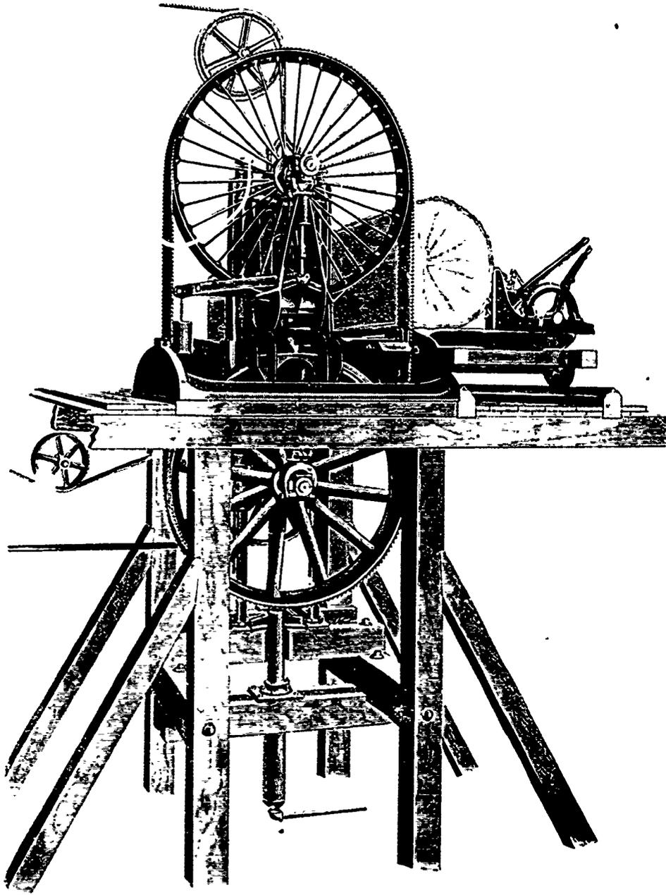
The machine is now, and has been for over seventy-five days, running twenty-two hours per day, fitted with double-toothed band saws, in the H. C. Akeley Lumber Co.'s mill at Minneapolis, Minn.
