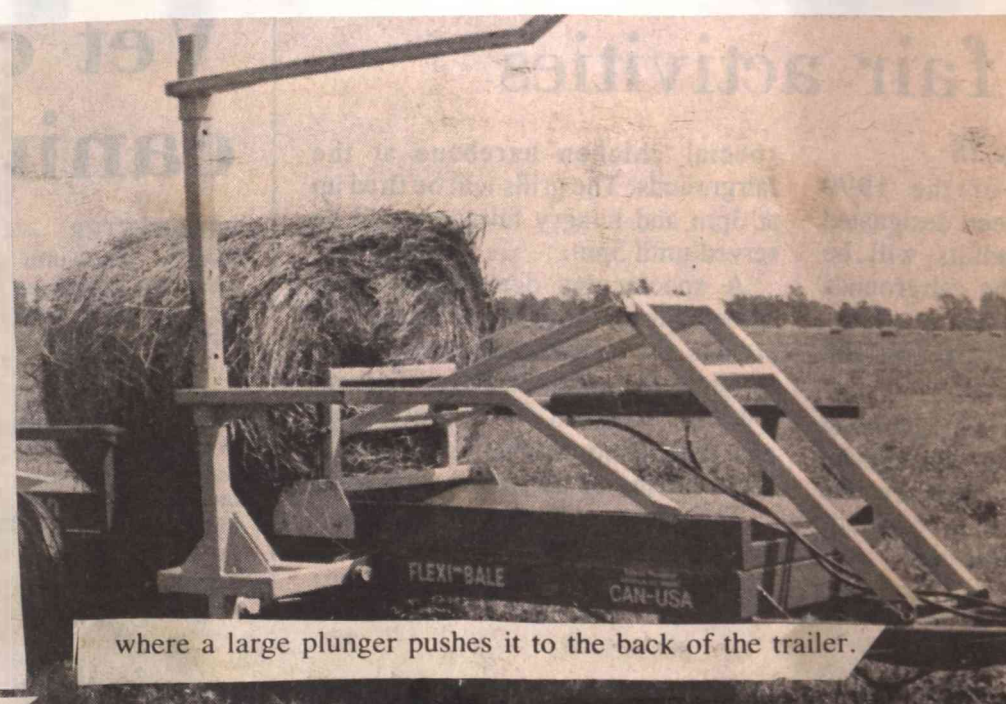
The Flexi-bale F-40 loads large round bales from the side;
