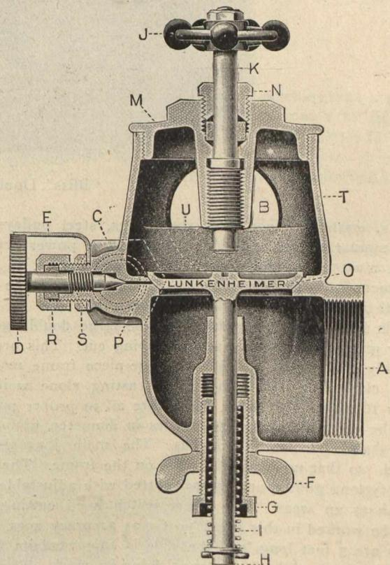
tension can only be ascertained by trial when the engine is running, the adjusting arrangement of the valve illustrated, will be found a great improvement. The lift of the disc is regulated by means of the stem K.
