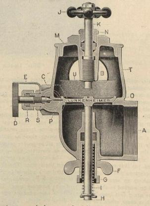
tension can only be ascertained by trial when the engine is running, the adjusting arrangement of the valve illustrated, will be found a great improvement. The lift of the disc isregulated by means of the stem K.
