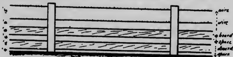
FIG 3 CEDAR BOARD & WIRE FENCE.
