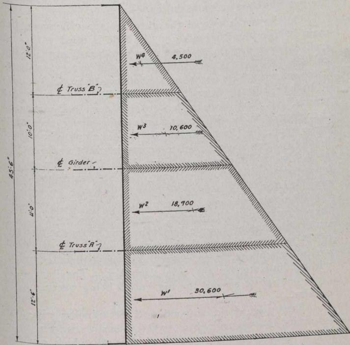
Fig. 2.—Hydrostatic Loading Against Rolling Caisson.
