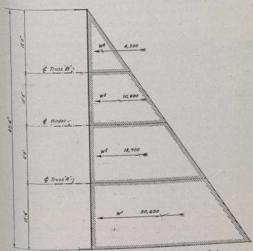
Fig. 2.-Hydrostatic Loading Against Rolling Caisson.
