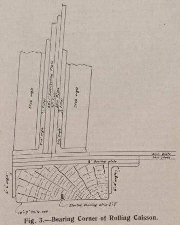
86,000 lbs. per square foot—600 lbs. per square inch which is even then very large for sill pressures. It was felt that, though the width of the caisson was fairly good (19 feet) the end itself would, owing to its construction, be hardly stiff enough to really distribute the highly con-
