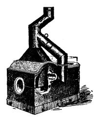
shown in the illustration. The heat arising in the main flue creates by induction a forced draft throughout the entire length of the muffle, the fresh air thus supplied furnishing abundance of oxygen, so that cupellation is both rapid and complete in all parts of the muffle.
