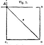
reach p in the same space of time that the force x would have sent it to B, and the force y would have sent it to c. Now, if two lines be drawn from n to join B and c, a square will be produced, and the oblique line e, which the body describes, is the diagonal of a square. Supposing
