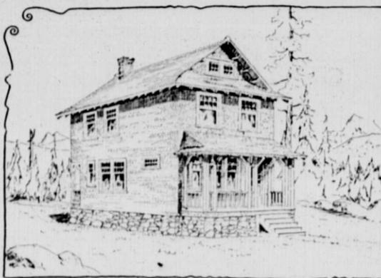
THIS ATTRACTIVE LITTLE HOUSE IS SHIPPED COMPLETE READY FOR ERECTION. ALL PARTS ARE MARKED CORRESPONDING WITH BLUE PRINTS, AND TALLY SHEETS SENT WITH SHIPMENT. ANY ORDINARY CARPENTER CAN ERECT IT.
