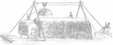
It is strong and simple, perfect working and durable, runs on  $_{5}\text{-8}$  inch steel cable uses either fork or slings, and builds any sized stack
