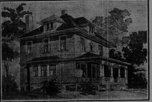
This design represents a house 30 feet front by 28 feet deep, exclusive of the piazat. The latter extends the full width of the front and is 9 feet wide. The exo ternal appearance of this house is sym-metrical, with the wide projected eaves and timber brackets on the under side, the treatment of of the piazza and main roof being the same. The cornice mem-bers of the piazza are carried around the house and the upper portion of the wails are shingled, while the first story is cov-
