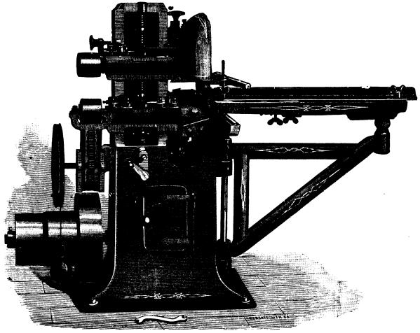
This is an entirely new style of Tenon Machine. The frame is cast in one piece, and the working parts stand solidly on a pedestal, avoiding vibration.
