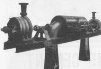
Two Worthington 3-Stage Turbine and McCormack Water Wheels, built for Port Arthur, Ont., Water Works, (440 gal. per minute against 350 ft. head. WATER WORKS SYSTEMS INSTALLED
